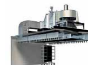
Thawing installation Page 36
